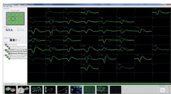
Screenshot of AxIS software showing waveforms of detected spikes
